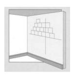
Dekwall should be installed as "Brick-Bond" layout Carefully place the central panel in position and press it gently, especially at the edges.
